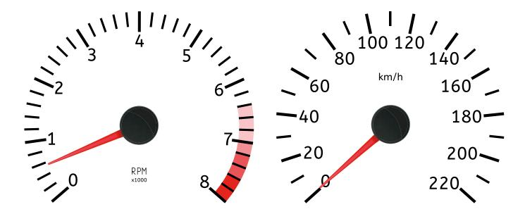
vehicle whose engine is running but in a neutral gear and stationary is at idle. The set point of that engine speed varies between manufacturers. For a Mercedes-Benz heavy-duty engine it's 500rpm (compared to a normal operational range of 900-2,200rpm); for the DAF MX-11 and MX-13 it's 525-600rpm; for Scania it's 550-650rpm, depending partly on ancillaries.
